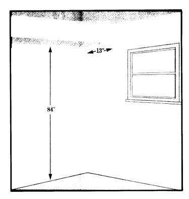
**Soffits:** A soffit is the bulkhead between the ceiling and the top of the cabinets. Distance from floor to soffit should be at least 84". (Allow 1/4" more if you install an 84" tall cabinet). Depth may vary. Normal is 13" - 1" deeper than a wall cabinet.
