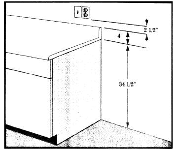
Base Clearance: You need 41" below windows and electrical wall outlets to fit in new base cabinets and a counter top with backsplash. This leaves 2 1/2" clearance above the counter top. If you have less than 1" clearance, consult your designer.
